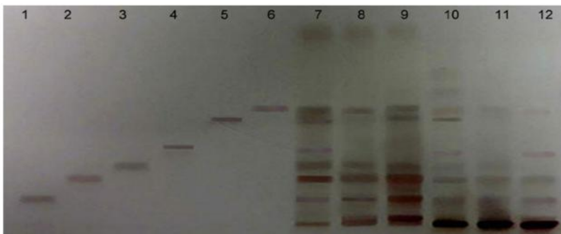
Fig. 6. HPTLC chromatogram for Withania somnifera (Ashwagandha). Visualization was made under UV light of wavelength 231 nm.
